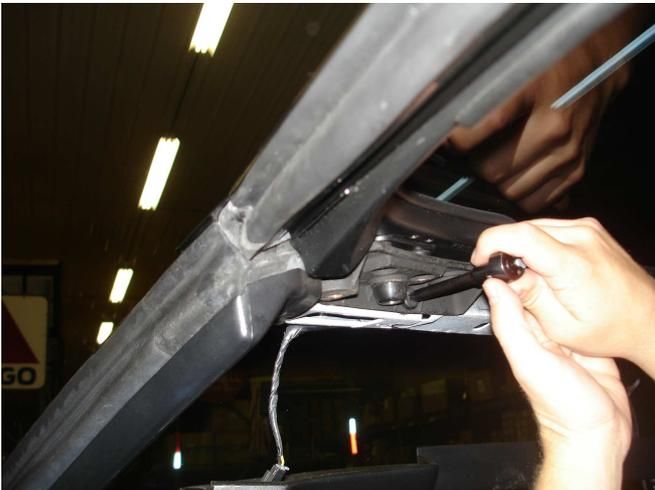
12. Once roof is adjusted reassemble trim parts in reverse order. Pay attention to rear view mirror wires so they don't get pinched.
