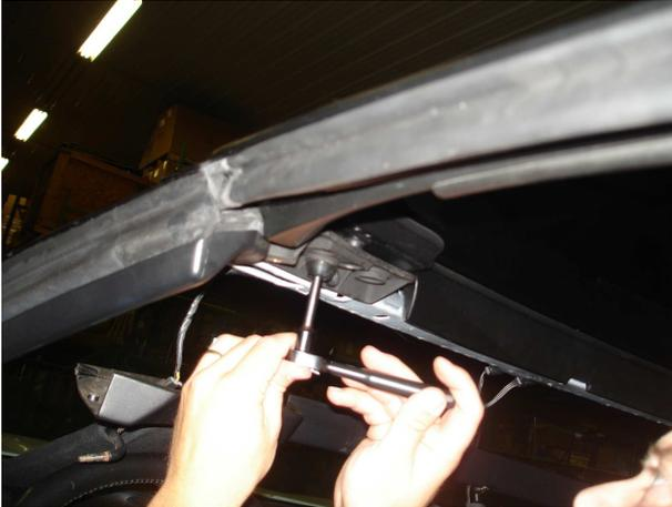
9. Tighten outer front roof plate bolts
